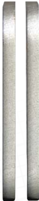
Example for ¼" (6mm) Aluminum cut with WMS
