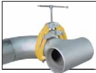
Fit-up 90° fitting to tee
