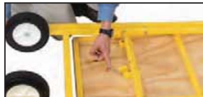
Plunger pin locks legs in open or folded position.
